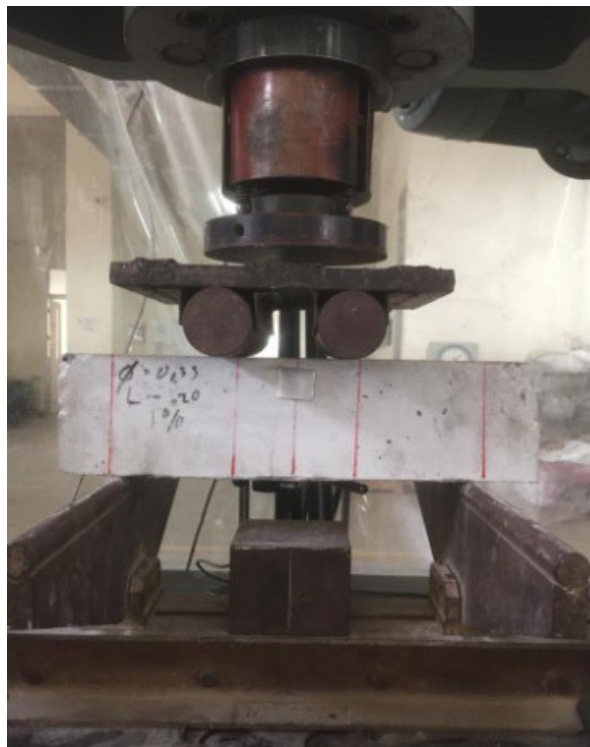
Figure 1. Flexural strength testing.
